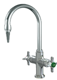
Deck Mounted Mixing Faucet Hot and cold water faucet. 6" gooseneck. 3/8" NPT. Cat. No. 50026 with vacuum breaker Cat. No. 50018
